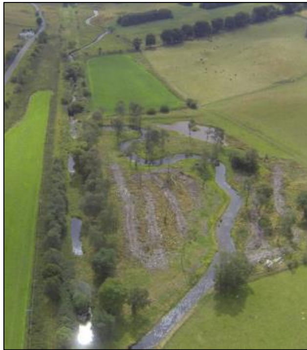
Figure 5-9 Re-meandering by the Eddleston Water Project (UK) (Source: amended from Tweed Forum for EA WWNP)
