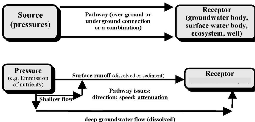
**Figure 1:** Pressure – pathway-receptor model for implementation of the WFD
