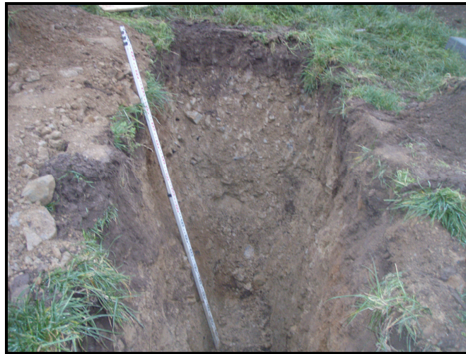
Plate 3. Trial hole, Site F. The well aerated topsoil material is visible and mottled and stiff to very stiff subsoil (photo: Robert Meehan).
