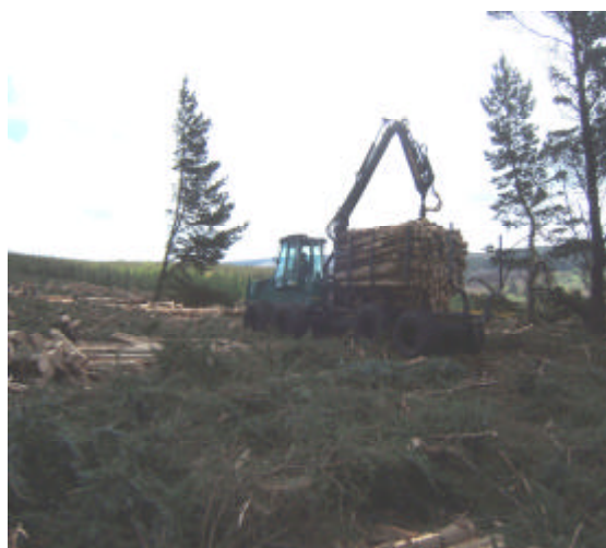
Figure 3 Forwarder removing timber from site
